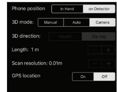
Camera mode is only available for GoldenEye & GoldenEye Plus detector model. In order to use this feature, smartphone must be placed on the handle that is mounted on detector and also Phone position must be set to "on Detector"
