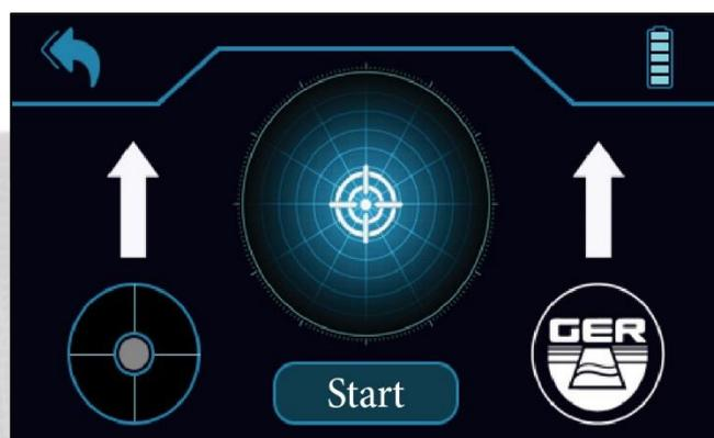
Turn in the opposite direction, press the start button, wait until you hear a beep emanating from the device, and the icon shifts from the rotation position to the forward position, then walk until the device rotates backwards, the device will analyze and show the final results automatically.
